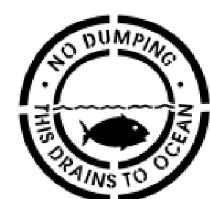
CATCH BASIN STENCILING SAMPLE S1 SCALE: NTS
