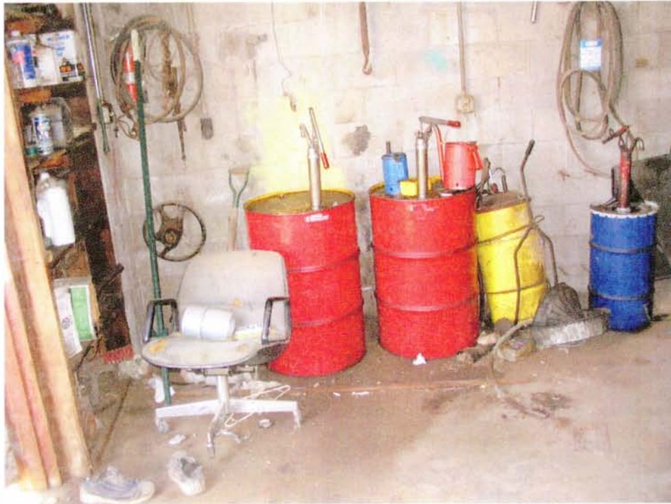
Drums of oil stored in barn. Note surficial oil staining on concrete.
