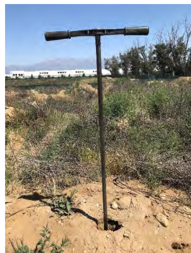
6. Hand auger soil boring SB-3 in the southwest portion of the piles of dumped soil/fill
