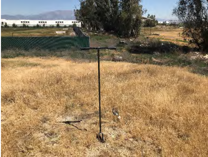
7. Hand auger soil boring SB-4 in the northeast portion of the piles of dumped soil/fill
