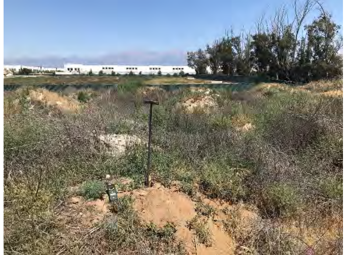
8. Hand auger soil boring SB-5 in the central portion of the piles of dumped soil/fill
